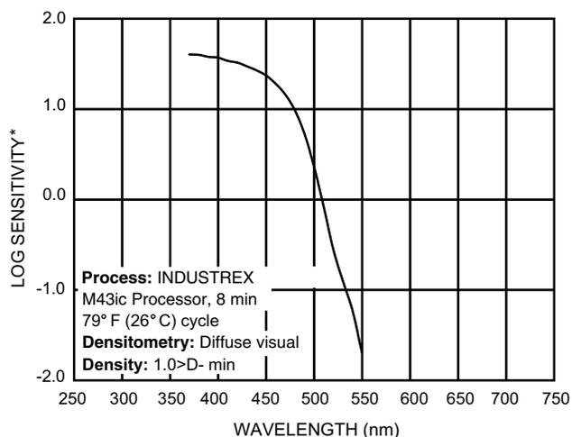
\*Sensitivity = reciprocal of exposure ( $\text{erg}/\text{cm}^2$ ) required to produce specified density
